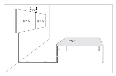
Note: If the cable length you required is more than 7 meters, USB extension cables can be used for wiring.
