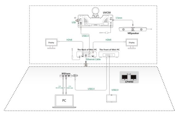
Note: For more information about the installation and deployment of accessories (for example, the installation of mini-PC package or UVC50 camera), refer to the Quick Start Guide of the corresponding accessory.
