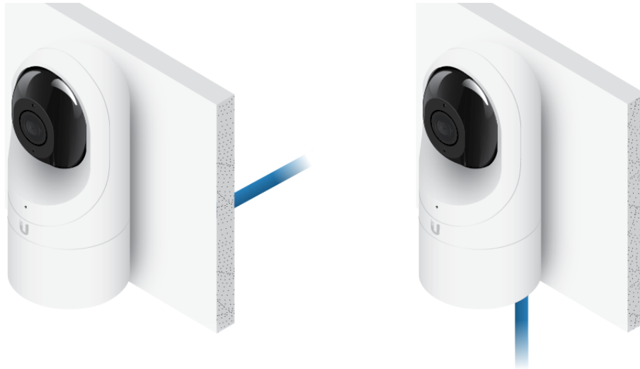
Indoor Wall with Flush Mount
