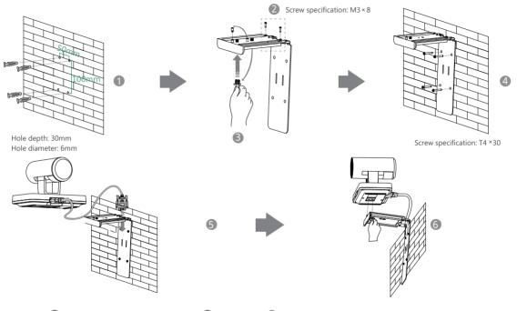
Steps: ① Punch holes & Insert expansion bolts ② Drive screws ③ Adjust the screws position and manually lock them ④ Insert screws to lock the bracket to the wall ⑤ Connect DVI cable ⑥ Lock the camera
