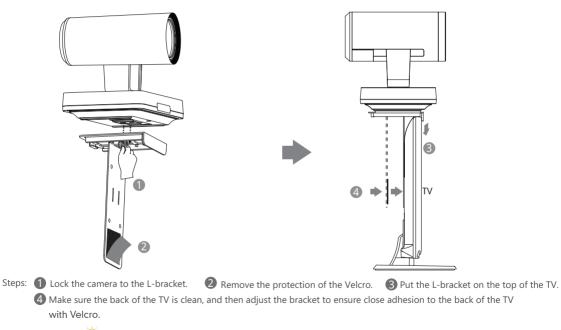
Adjust the bracket to ensure close adhesion to the back of the TV
