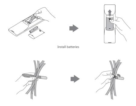
Fasten the cables with the cable tie
