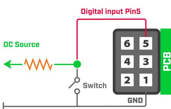
**note:** Digital input voltage is 0-2.5 V max.
