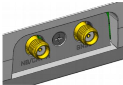
**i** BG77 supports NB and GNSS. Both cannot be used together simultaneously. Please check the guide at - [WWAN and GNSS priority automatization](#).
