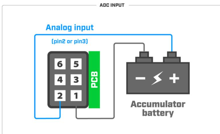
**note:** Analog input voltage is 0-60 V. Theoretical resolution is 4 mV (14bit ADC). Analog input impedance is approximately 72K Ohm.
