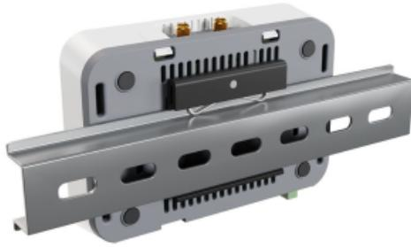
1. The device can be mounted using provided DIN rail mount set. Designed to fit standard 35 mm x 7.5 mm DIN rails. Attach it with two provided screws to the device and attach the device to the DIN rail. The DIN rail is not provided in the package.
