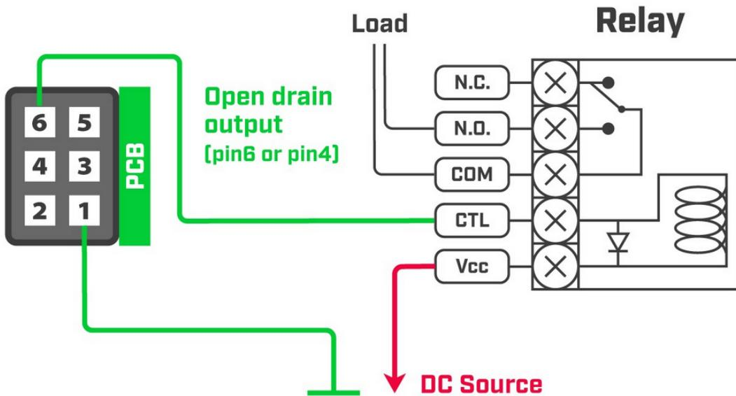
**note:** The maximum power dissipation (for digital output open drain transistor) is 0.48 W, and the maximum voltage is 30 V or 2.8 A. For example 0.48W / 1V = 0.48A, or 0.48W / 2V = 0.24A etc.
