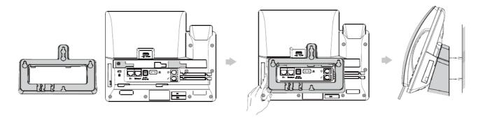
Note: The reversible tab has a lip which allows the handset to stay on-hook when the IP phone is mounted vertically. For more information, refer to Yealink Wall Mount Quick Installation Guide for Yealink IP Phones.
