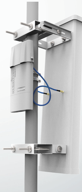
Using the optionally available Flexguide cable, you can use the Basebox with any 3rd party antenna
