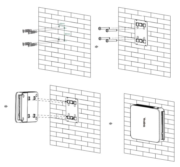
Before mounting the bracket, you need to confirm the direction of the MCore installation. Once the bracket is mounted, the installation direction of the MCore cannot be changed.
